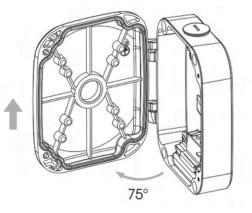
Step 2: Loosen the screws of the fix rings, put rings through the back of the box body;
