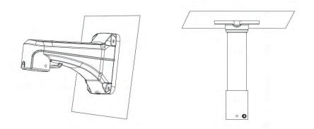
Step3: Put the cables through the holder. Match the holder with the screw holes of the camera body and secure them;
