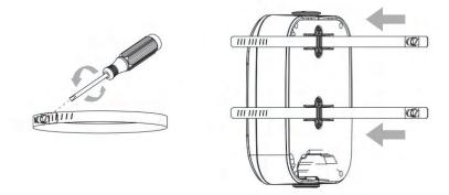
Step 3: Fix the rings with rear cover on the pole, fasten the screws;
