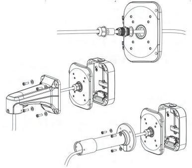
Step 8: The box supports top or bottom cable-out ways as below picture, through the top hole, or tension disc which put cables through bottom or bottom back. For tension disc, please remove it then cut an opening on the rubber plug, get cables through the opening. Please remember to plug the rubber plug whenever the holes on it are not in use;
