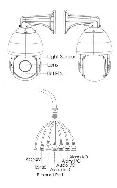
NOTE: 1) Only AC 24V is available for Speed Dome Network Camera power supply. AC 24V and PoE+ (802.3at) are available for PoE Speed Dome Network Camera power supply;
